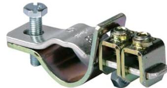
The earthing terminal AM8 is mainly used for connecting the earthing conductors to various pipework in sizes Ø 8 - 28 mm. It is possible to adjust the terminal to suit to four different pipe thicknesses. The terminal has two 35 mm<sup>2</sup> pillar terminals. The conductor bar is made of tinned copper and the strap of zinc-plated steel. The pillar terminals are of zinc-plated and yellow passivated steel.
