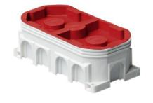
The box AU17.2 has knock-outs for 11 inlets on the side, and 6 on the bottom. It can accommodate a device with a triple inlet. If necessary, the box may be divided in two by using partition plate PMR345. Made of halogen free material (IEC/61249-2-21) and fulfills the requirements of the glow wire test according to the standard IEC/EN60670: 2005 (850 °C).
