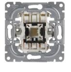
Control switch insert without rocker. All 1-gang rockers fit to the insert, but in control switch use the rocker 1788-xx must be used. The switch insert has separate circuit-breakers for the N- and L-wires and 2 Xterminals. The X-terminals can be used for extending other wires. The signal light can only be set as a search- or signal light, but in control use it must be set as a signal light.
