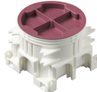
Mounting box for hollow wall installations and concrete casting walls. Box height is 59 mm and there is plenty of space for electrical installations. Several screw towers for easy and flexible socket outlet/switch installation with 60 mm screw c/c distance. Also box has longer screws compared to previous versions to give more flexibility in the installations.
