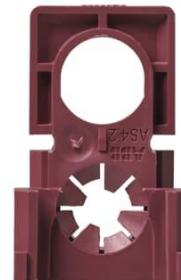
Multifunctional accessory for AU4.2 mounting box. It can be used as strain relief inlet, interconnector for c/c 71mm combinations and as box support for 66 mm frame. Also you are able to use two of them together for 95 mm frame box support.
